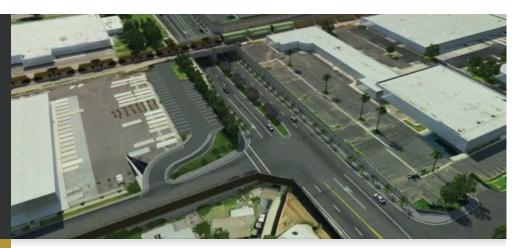
The City of Fullerton and the Orange County Transportation Authority (OCTA) are constructing a vehicle undercrossing at the intersection of State College Boulevard and the Burlington Northern Santa Fe Railway. The roadway is being lowered between Santa Fe Avenue to the north to approximately 500 feet south of Valencia Drive to the south.
